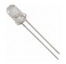
An LED bulb changes the electrical energy into light.
